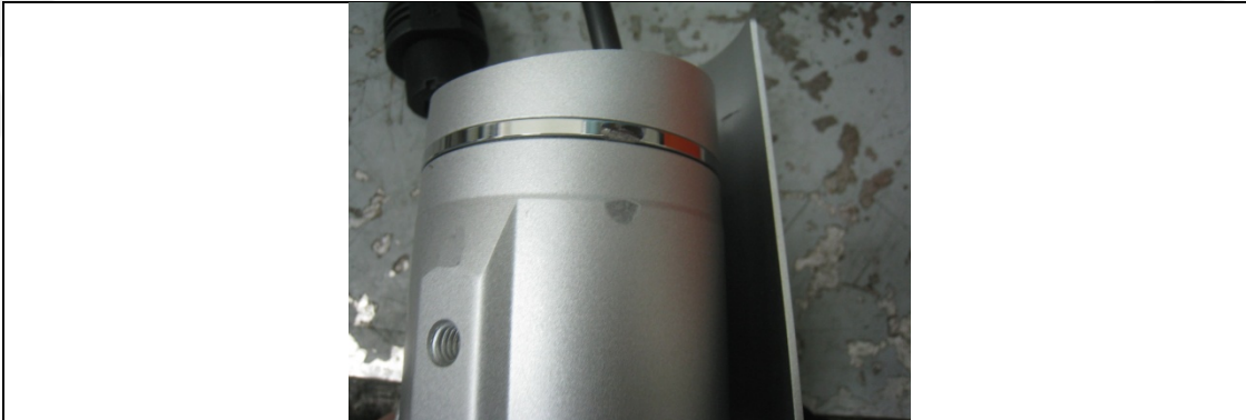
7. The cover of specimen deformed after this test (Position 3)
