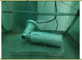
Test for protection against solid foreign 6. objects (Dust test)
