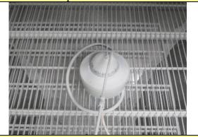
5. Test for protection against solid foreign objects (Dust test)
